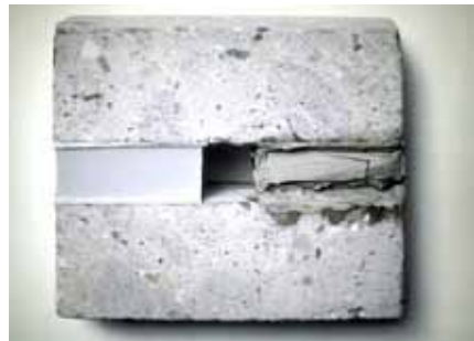
Dow Corning® silicone sealant (left) and a leading polyurethane sealant after 2,500 hours of humidity and UV exposure in extended weathering, heat and stability tests
