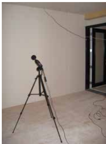
(a) Source room with an omnidirectional loudspeaker as the source and a sound level meter (b) Receiving room with a sound level meter to measure the sound transmitted through the wall
