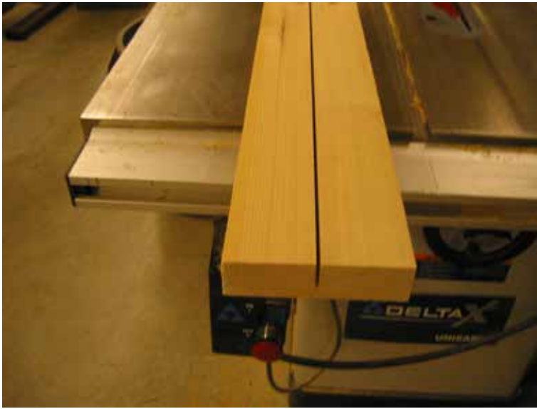
Figure 3 Lumber shrinkage relief
