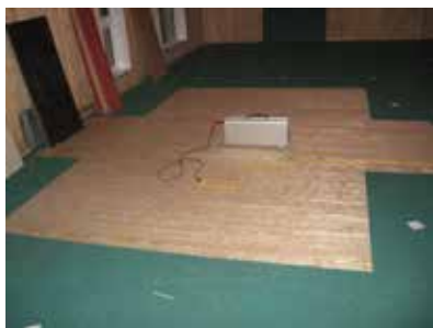
(a) Source room with the tapping machine on the floor in a field floor/ceiling assembly
