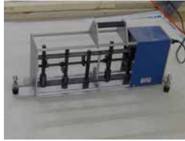
(a) Acoustic chamber showing the floor specimen and tapping machine (b) ISO tapping machine
