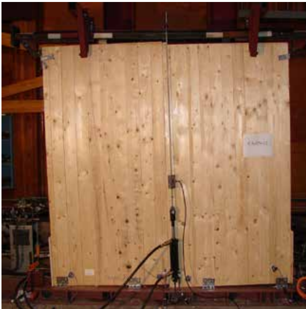
Figure 3 Rocking behavior of a two-panel CLT wall during testing (FPInnovations)
