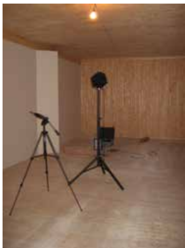
(a) Source room with an omnidirectional loudspeaker as the source and a sound level meter (b) Receiving room with a sound level meter to measure the sound transmitted through the wall
