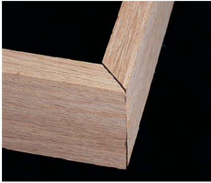
Avoid: mitered seat joints. They are not as strong and can open.
