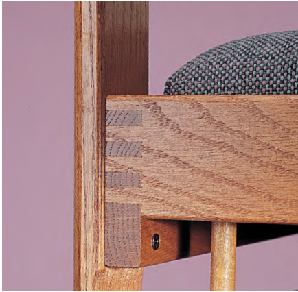
Avoid: seat joints that have only glue and screws. Although this has a strong finger joint at the seat corner, the stress point between the seat frame and the back leg is still only glued and screwed together.
