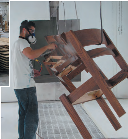
After hand staining, New Holland's craftsmen apply a vinyl sealer and then a top coat.
