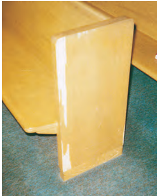
Avoid: a poorly manufactured end panel which may result in delamination of the veneer.
