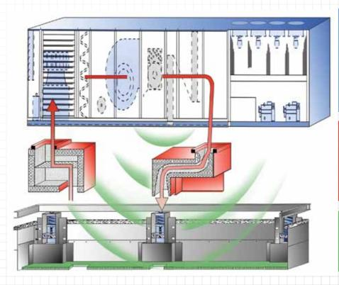
Vibration from fans and compressors (source 1) and vibration from casingradiated noise caused by duct turbulence and the airborne noise of the fans and compressors (source 2) are controlled with Kinetics high deflection, laterally stable coil spring isolators and high frequency neoprene noise pads.
