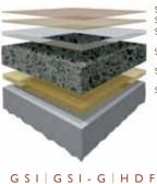
Stonseal Sealer Stonkote CE4 Stonblend Groutcoat Stonblend Mortar Stonhard Primer Substrate
