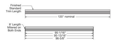
Test one piece of trim running the length of install to make sure the FXTBC clips are positioned correctly (measurement from T-Bar hook flange to cross tee should be 23-1/16" – standard 2' x 2' grid opening).
