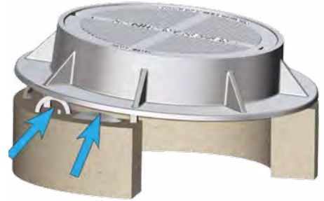
Water penetrates shimming material and through cavities.
