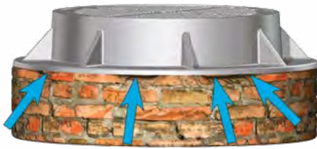
Water penetrates between rigid and irregular surfaces.
