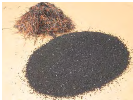
Crumb rubber recycled from old tires and RFL coated fiber.
