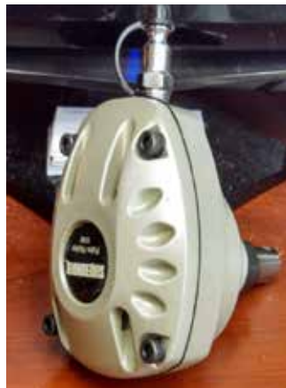
SUREBONDER 9760 Hand Held Nail Gun - Used on individual nails not driven flush with picket. Hold nail gun over nail, insert over head of nail, and drive nail to be flush with surface of fence panel. Available in most homecenter stores.
