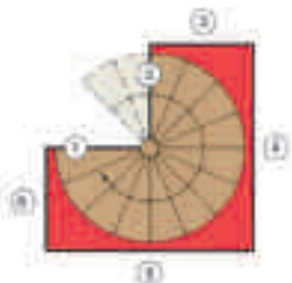
Left Hand Up Standard 22 1/2° 16 Treads per circle Riser height 6 1/2" to 7"
