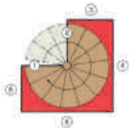
Left Hand Up Standard 27° 13 1/2 Treads per circle Riser height 7 1/2" to 8"
