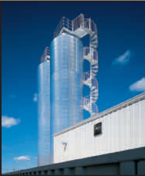
60S 56' floor to floor, 1-1/2" Rd. handrail, 1" square balusters, checker plate treads, 60" rest landings
