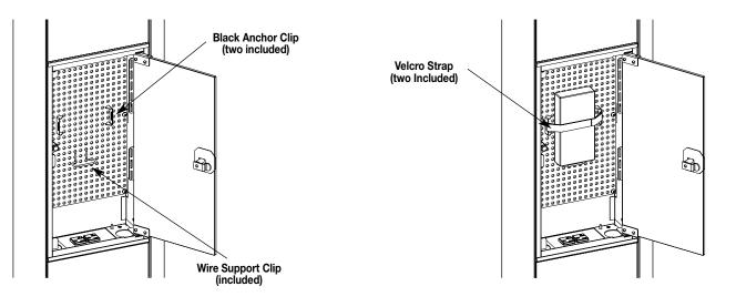
**Device installation using Support Clip and Side Rails**
