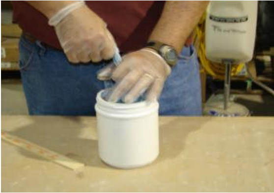
Mix resin and catalyst
