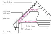
Upon completing steps 1–3, proceed to steps 4 & 5. Working toward the peak of the roof, continue to place and staple subsequent *raft-R-mate* vents between rafters. If a full length vent will not fit, overlap or cut one to fit remaining space. *raft-R-mate* attic
