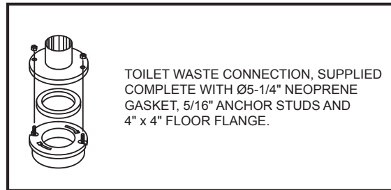
(TW4) FLOOR OUTLET WASTE CONNECTION
