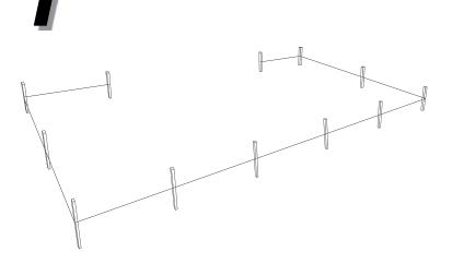
Dig post holes 12" in diameter 36" deep. Use the Center to Center measurements of the fence model being installed for the Center to Center Post Distance.
