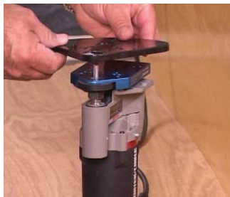
STEP 1 Attach the plate.
