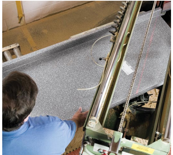
Precision countertop saws used in fabrication are easily adjusted to any angle for cutting miters that have a professional fit.
