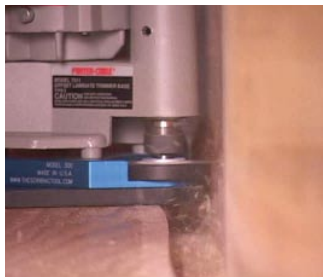
STEP 2 With the countertop fastened less than one inch from the wall, the router does the cutting.
