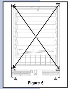
right hand opening. The door opening is easily reversed by moving the hinge hardware to the opposite side (see Figure 6).
