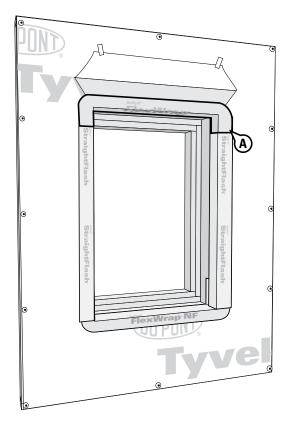
After the outside portion of the recessed opening has been integrated with the WRB using DuPont<sup>™</sup> FlexWrap<sup>™</sup> NF, and DuPont<sup>™</sup> StraightFlash<sup>™</sup>. The remaining rough opening should be coated using DuPont<sup>™</sup> Tyvek<sup>®</sup> Fluid Applied – Brush Formulation. Before beginning be sure to clean surface of any loose material or debris that may affect adhesion of the Fluid Applied product.
