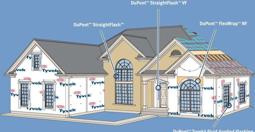
DuPont™ Tyvek® Fluid Applied Flashing – Brush Formulation
