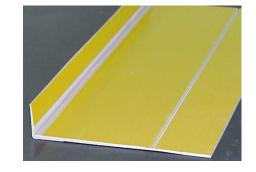
Next, apply one length of the 9-1/2" wide strip of Power Tape approximately 1/2" back from the internal angle of the stair tread nose and another length of Power Tape across the riser portion of the stair tread, as illustrated. Thoroughly roll the tape to ensure proper bonding to the back and nosing areas of the stair tread. Trim off excess Power Tape along the edges of the stair tread as required.
