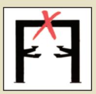
Mohawk two post lifts use height adjustable overhead stainless steel hydraulic lines NOT restrictive overhead cable and rubber hose covers that limit lifting height.
