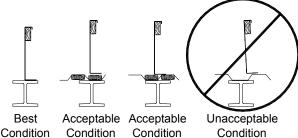
As an alternative, the roof curb can also be mounted on a roof deck. When a deck is used, be sure to provide additional blocking directly below the curb flanges to give further support and minimize vibration. (See below)
