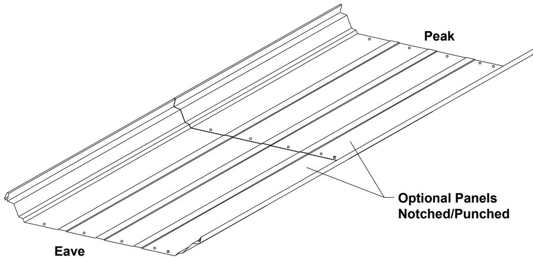
**Factory Notched / Punched Panels** - Unless otherwise specified, Metal Sales provides all Snap-Loc 24 panels with no factory rib notching or fastener hole punching. **Panels that are to be factory notched/punched must be specified at time of order.**
