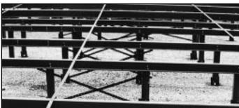
ASTM A570 grade 55 steel (55,000 PSI minimum yield point) finished with a red oxide or G-90 galvanized finish (which meets ASTM A653). Cee or Zee shapes with web depths of 4", 6", 8", 10", and 12" with a variety of symmetrical or unsymmetrical flanges available. Special shape, single or double slope and high or low side struts are available up to 40'-0" lengths.
