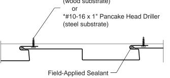
\*Pre-drilling into thicker steel may be required.
