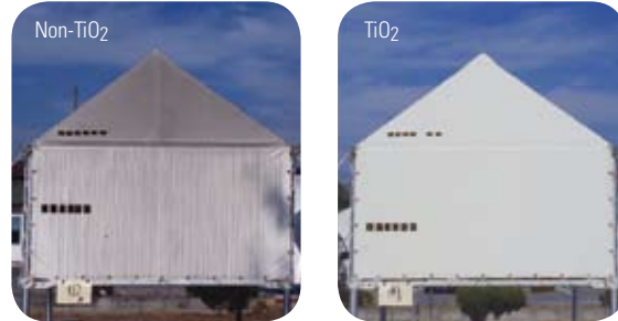
PVC coated fabric after 5 months outdoor (Saitama, Japan)
