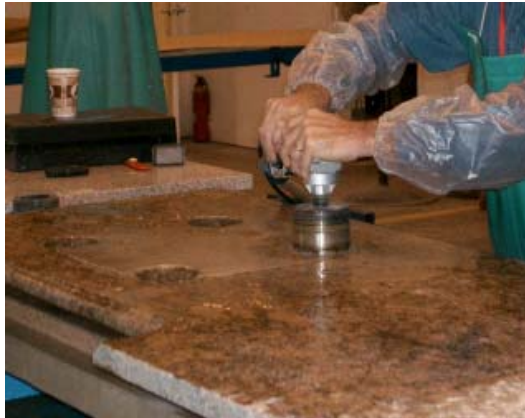
Wet drilling with core bit
