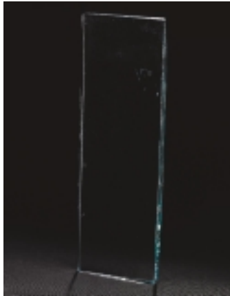
After testing in the Cleveland Condensation chamber, uncoated clear glass had a hazing reading of less than 1 percent.
