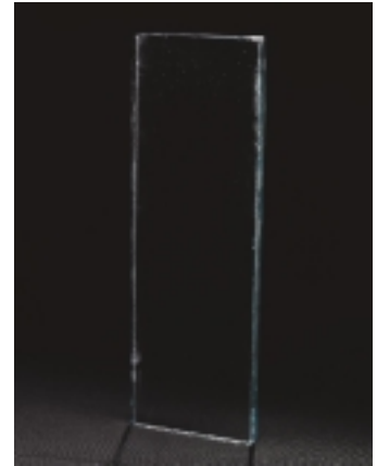
The haze reading for Clarvista glass in a clear glass substrate was less than 1 percent after Cleveland Condensation testing.
