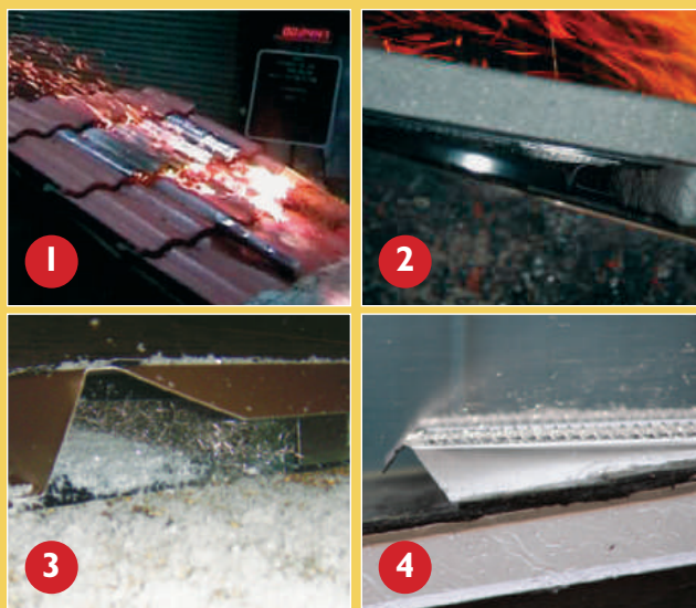
1. Flame and ember test performed on all O'Hagin's FIRE & ICE™ Vent profiles; 2. Cut-away side view of batten cavity during flame and ember test illustrating vent resistance to flame and ember penetration into batten cavity and interior attic space; 3. Photo of O'Hagin's new FIRE & ICE™ Tapered Low-Profile Vent taken during wind-driven snow demonstration in the Sierra Nevada at 7,200 ft. elevation — illustrating protection of airway from snow intrusion or build-up by patent-pending stainless-steel matrix while providing superior airflow; 4. Tapered Low-Profile FIRE & ICE™ Vent during FBC TAS 100(A)-95 Attic Vent Testing for wind-driven rain and snow.
