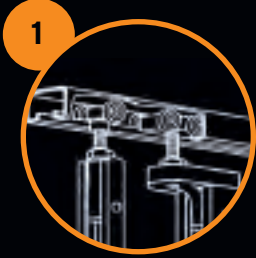
Adjustable ball bearing trucks in box type tracks for smooth operation, 2-wheel trucks on intermediate.
