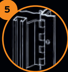
8" seven knuckle gate hinge. 0.1875" leaf, 0.4375" pin, mortised into Z bar frame. Offset hinge permits cabinet doors to close with gate in either position.
