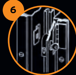
0.1875" thick cold-rolled facia strip and door on deep type cabinets for adequate strength and better finished appearance.
