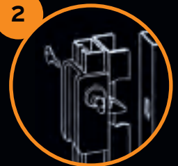
Cylinder locks mortised into gate end bar. Keyed both sides. Yale mortise cylinders, or master-keyed to building system.
