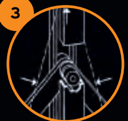
Machined roller bearings in all vertical channels assure ease of operation, proportionate spacing of lattice bars.
