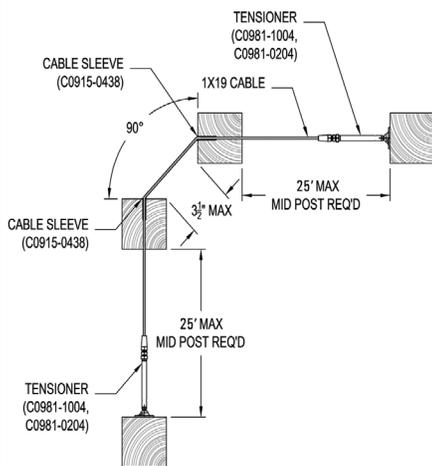
Follow the recommended tensioning sequence below to ensure proper installation and to achieve optimal results.
