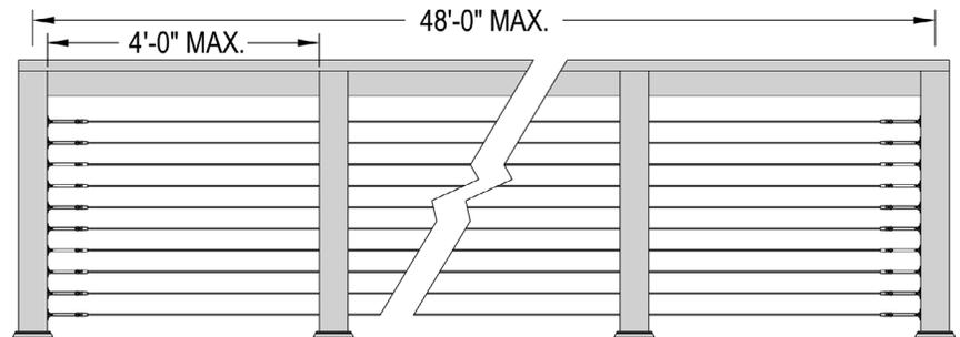
For straight cable sections using the RailEasy™ Tensioner at each end, you may run cable up to 48 feet in total length (mid post required as specified).
