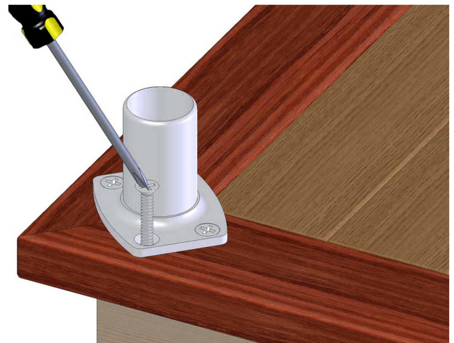
Figure B. Fasten each base to the deck with four (4) screws.
