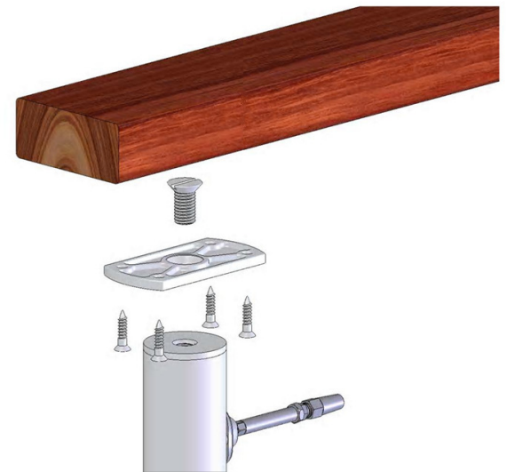
Figure C. Fasten the top rail using the provided wood screws.
