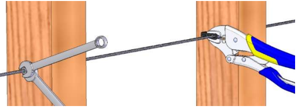
Figure H. Use a cable grip pad with vice grips to hold the cable tight.
