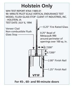
\*NOTE: Wood beads for use on VT's 5-ply wood veneer mineral core doors (45-, 60- and 90-minute) are made of an incombustible material, veneer wrapped to match the wood veneer door face. Not for use on HPDL doors.
