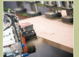
Pre-drilled pilot holes provide ease of installation.
