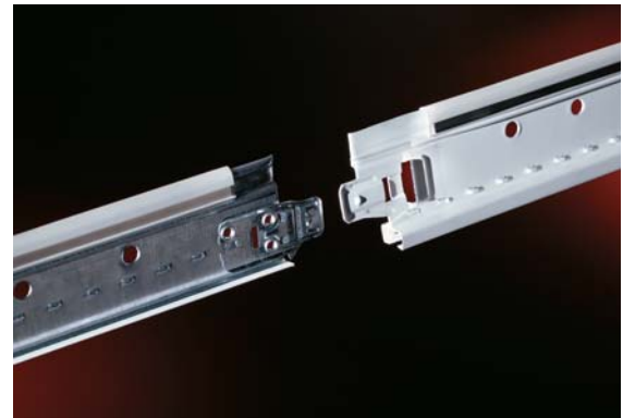
Suprafine DC Main Beam (left); Silhouette DC Main Beam (right) Electrical conductors are embedded on the top of each type of grid main. Silhouette has conductors embedded in the bottom slot also.
