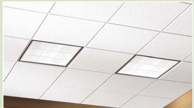
2' x 2' ceiling panels on Suprafine DC Grid Lay-in light fixtures can be powered directly from the ceiling grid, with no hard wiring, and can be quickly and easily moved when needed.
