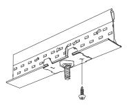
All single cross tee insertions must use the ARPLUG to lock the cross tee to the outside main beam
