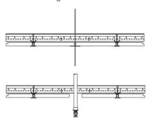
**6.5.2.** Notched Panel for Penetration – If the obstruction or penetration prevents the panel from fitting over it, you will need to notch the panel to fit around the penetration; e.g., structural brace, roof drain line, hangers for other services.
