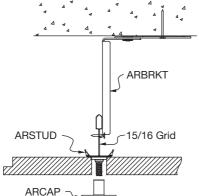
Optima Capz panels have Reverse Tegular edges. Panels are pre-drilled to accept hardware caps. Hardware caps attach to threaded studs which clip onto the suspension system. Unlike many conventional lay-in ceiling products, the Optima Capz edge detail does not lay into the suspension system.
