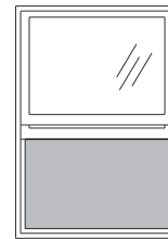
Shaded portion shows vent area.
