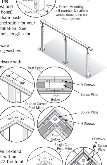
**5) Fasten Top Rails:** Secure the top rail to each post using two H screws (four screws for butt splices); screws should run through the top rail flange and into the post face. Attach screws to both the front and back of each post.
