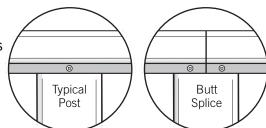
**5A)** Cut & Attach Wood/Composite Cap Rails (for Series-400 Top Rails only):
