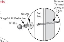
Using a 7/16" wrench, tighten the Snug-Grip® washer nuts until the cables are taut. Hold the shaft of the Threaded Terminal with Vise-grip® pliers while tightening.
