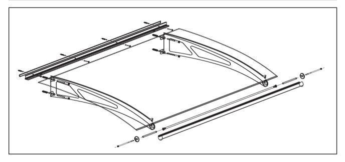
Lightline canopy kits come with all the hardware needed to assemble. Please verify what type of wall you are dealing with before installing the canopy. If necessary, you may need to use screws and anchors other than those included in the enclosed installation kit. Consult a licensed contractor for installation hardware recommendations.
