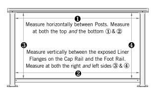
Note: Calculate Actual Glass Dimensions: If you are providing your own glass, calculate the actual glass panel dimensions by taking the measurements as described in step 11 and deducting 3 inches from your horizontal measurement and adding 3/4 inch to your vertical measurement. Be sure to have the two vertical edges of each panel ground smooth to remove the sharp edges and prevent the chance of someone cutting themselves during installation.
