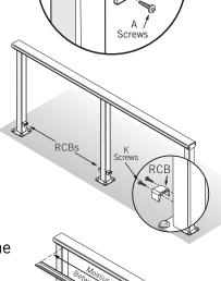
10) Install Foot Rails and Cap Infill Channels:
