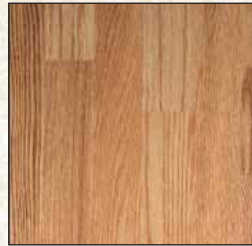
Red Oak Clear, Clear Quartered, Select Quartered, Select, No. 1 Common, No. 2 Common, and Rustic
