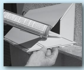
The basic bird deterrent slope, without an extender can treat a ledge 6" wide, there are extenders that can be attached for ledges up to 10" wide.
