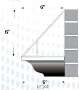
Ledges: Bird Slope mounted on a ledge turns it into an area that pest birds cannot land. Creates a "slippery slope".
