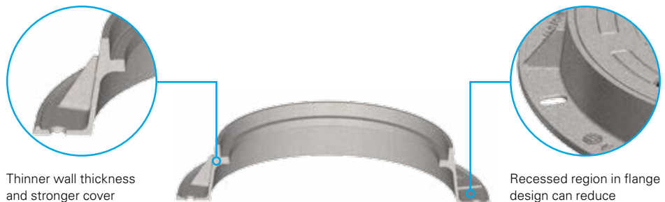
Ribbed modern cover design for ductile iron
