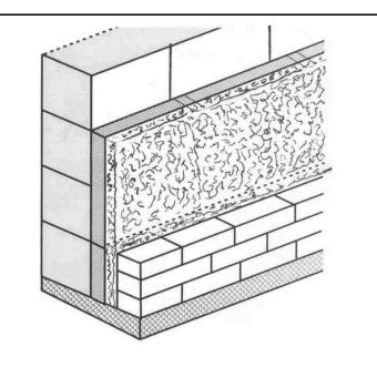
Install subsequent rows of CavClear prior to exterior masonry work.
