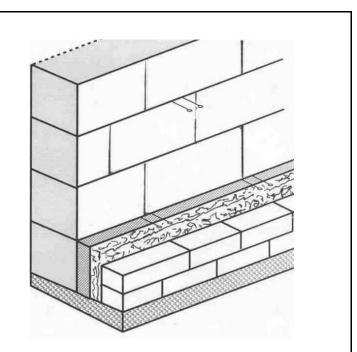
Do not construct exterior wythe to first set of ties until after first row of CavClear is installed.
