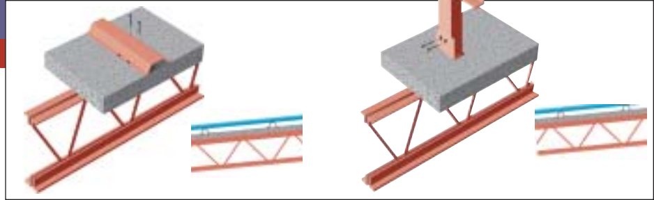
Hat section purlins over an existing structural system that run parallel to the roof slope. Existing roof slope to be maintained.
