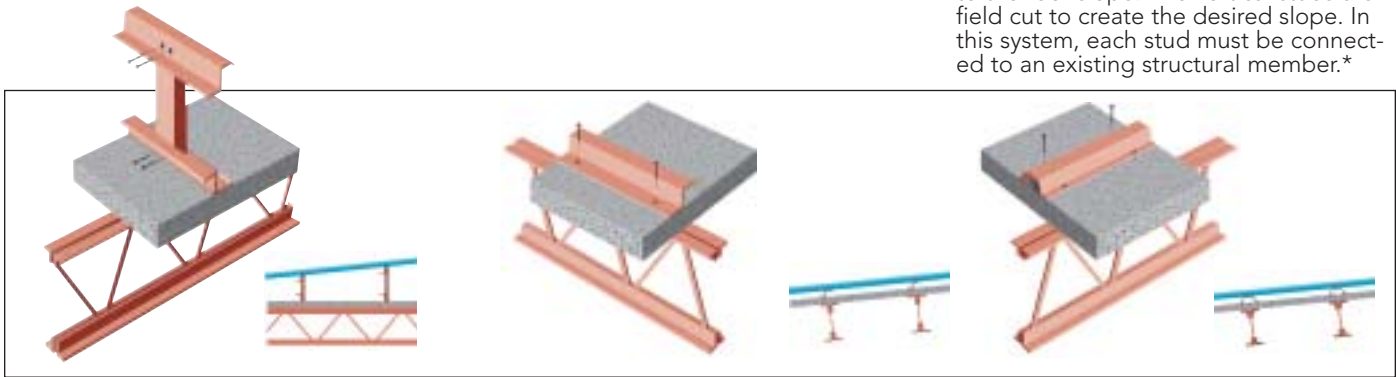
Roof slope buildup using zee base runners over existing framing running parallel with the roof slope.
