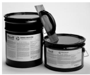
**E-Grip II**<sup>™</sup> is a low VOC, one-component urethane adhesive with excellent trowelability and superior tack properties. It is formulated specifically for use with Dodge-Regupol recycled rubber flooring systems. **E-Grip II** is a moisture cured, non-sag, permanently elastic adhesive that has excellent adhesion to elastomers, concrete and wood and is engineered for
