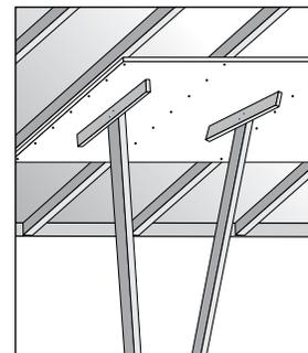
1/2" (12.7 mm) DensArmor Plus® may be applied to 24" (610 mm) o.c. joists as long as it is installed across or perpendicular to ceiling joists as shown.
