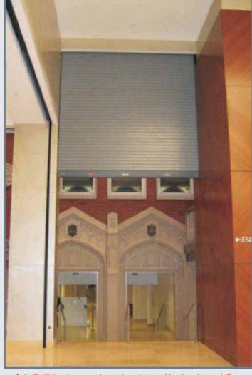
Auto-Set® fire doors can be custom designed to almost any width or height allowing for the needed design flexibility
