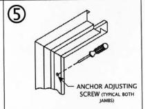
TURN ADJUSTING SCREWS IN BOTH JAMBS COUNTERCLOCKWISE UNTIL ANCHOR IS RESTING AGAINST THE WALL.
