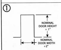
ADD TO DOOR OPENING DIMENSIONS: 2" TO WIDTH AND 1" TO HEIGHT. FOR A 3068 DOOR FRAME, THE ROUGH OPENING IS 38" X 81".
