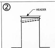
INSTALL HEADER INTO POSITION APPROX. 1" FROM TOP AND IN THE CENTER OF THE ROUGH OPENING.
