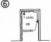
IF FEASIBLE, HANG DOOR NOW AND ADJUST FRAME ON WALL TO ALLOW PROPER DOOR FRAME CLEARANCES OR PLUMB FRAME WITH CARPENTER SQUARE AND/OR LEVEL. (ADJUST HEADER LEVELNESS BY SHIMMING UNDER JAMBS.)
