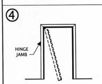
REPEAT STEP #3 WITH HINGE JAMB. PULL HEADER DOWN TIGHTLY ONTO JAMBS. LOCK HEADER AND JAMB TOGETHER BY BENDING OVER EXPOSED TABS.
