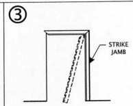
INSTALL STRIKE JAMB BY SLIDING OVER WALL AT TOP AND ENGAGING CORNER REINFORCING INTO HEADER. PIVOT JAMB INTO PLACE.
