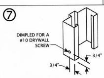
CHECK DOOR OPENING DIMENSION AT BASE OF FRAME (SAME DIMENSION AS BETWEEN JAMBS AT HEADER.) SECURE
