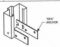
CHECK DOOR OPENING DIMENSION AT BASE OF FRAME (SAME DIMENSION AS BETWEEN JAMBS AT HEADER.) SECURE JAMBS
