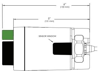
3. When the user steps away from the infrared sensor, the circuit initiates the flushing cycle to flush the fixture. The circuit then automatically resets and is ready for the next user.
